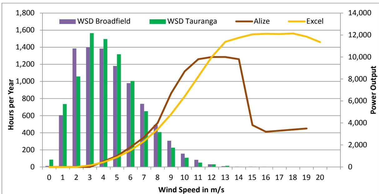
In Figure 21, power output curves of two SMWT with a capacity of 10 kW are compared and contrasted against the wind speed distribution.
