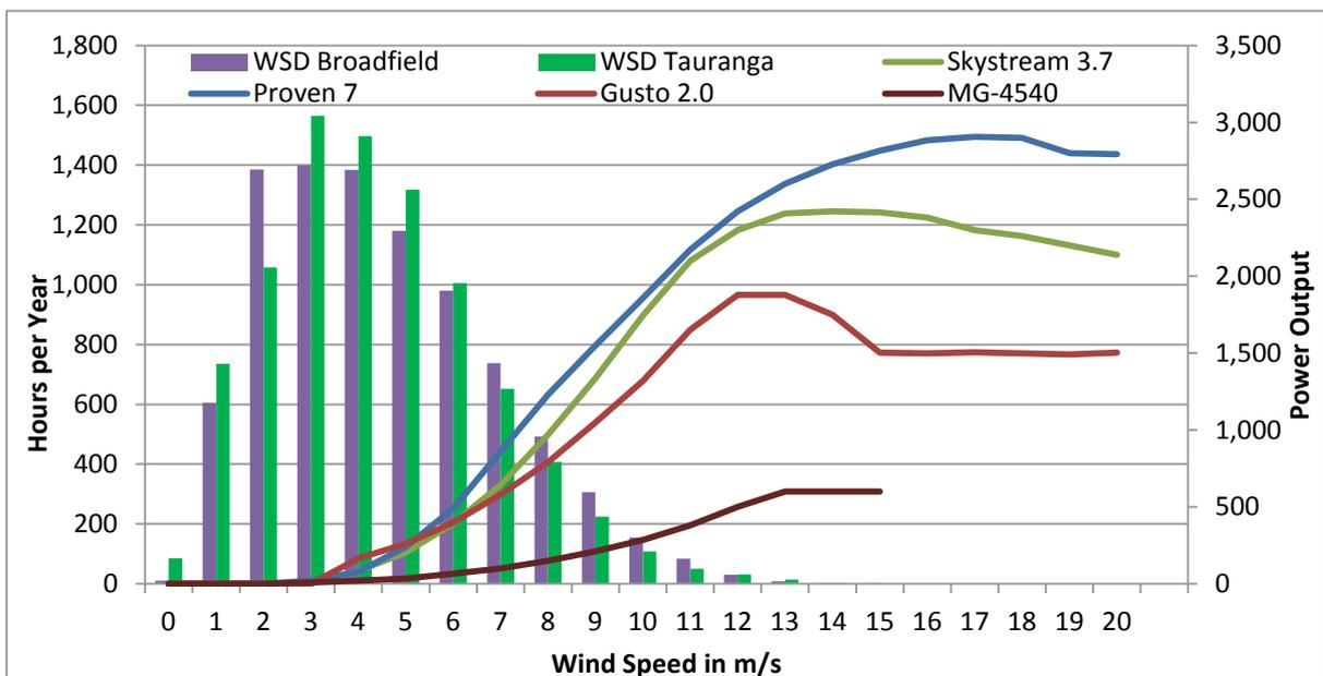
In Figure 20, power output curves of three SMWT with a capacity between 2.6kW and 6kW are compared and contrasted against the wind speed distribution.
