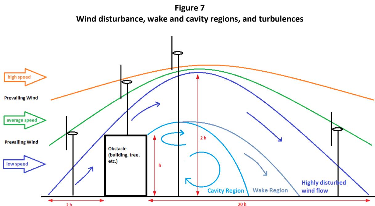
Disturbed regions (blue) normally range from two times the obstacle height before the obstruction and twenty times the obstacle height behind the obstruction. The height of these zones can be up to two times the height of the obstruction (EECA, 2010a). In this zone, the obstacle causes upstream
