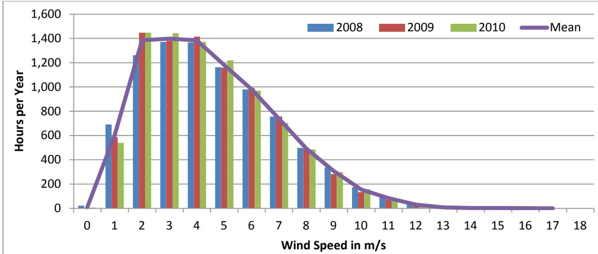
Figure 18 shows the wind speed distribution between 2008 and 2010 for the WBoP case study. Some inconsistency is noticeable at wind speeds between 0 and 2 m/s which may be due to a change in data acquisition in 2010.
