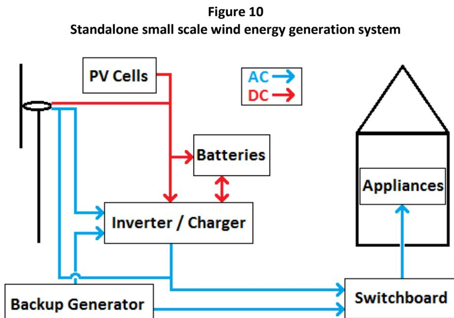
For standalone application, battery storage, generators and/or another kind of renewable generation systems (e.g. PV panels) are generally used to back up a SMWT (Gipe, 2004; EECA, 2010a):
