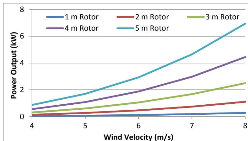
Figure 5 describes the influence of wind velocity and rotor diameter on performance of SMWT. In theory, doubling the blade diameter results in a fourfold of power output as the output increases by a square factor. Doubling the wind speed results in an eightfold of power output as the output
