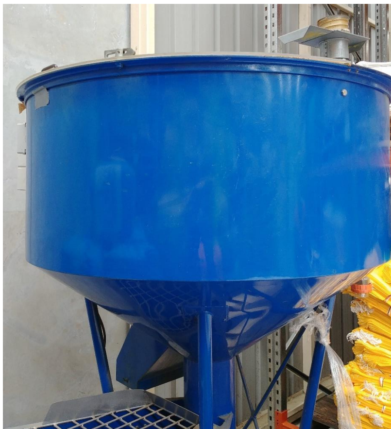
Figure 2.11 Custom made seed mixer used to add water to increase the seed moisture of the seed used in Objective 3.
