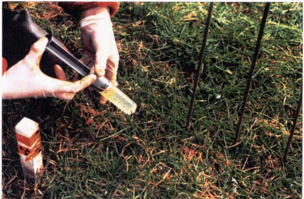
Plate 5.1: Injection of molten vaseline into the cavity left by the access tube from the microplots.
