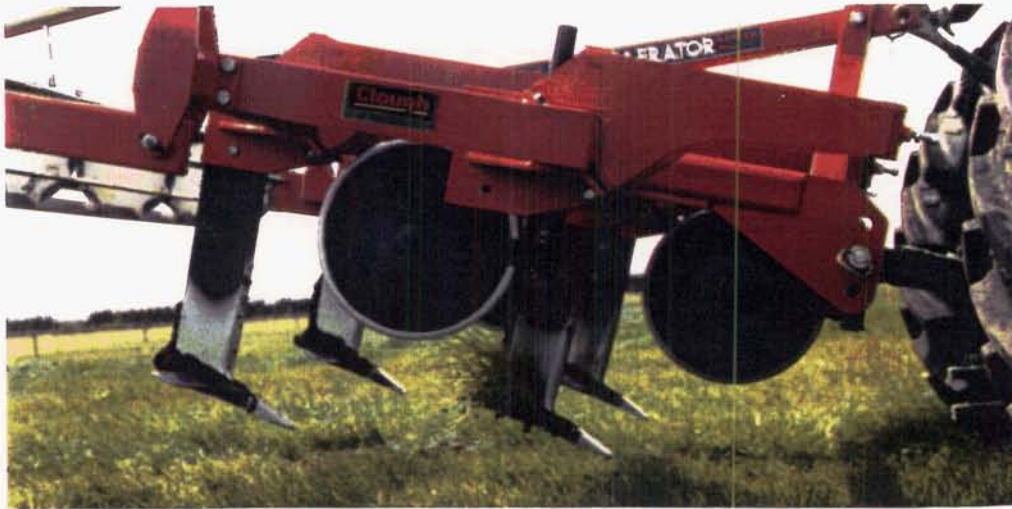
Plate 3.1: The Clough Panaerator used to aerate the profile to an average depth of 27 cm.
