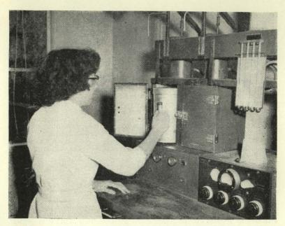
Fig. 4—Placing an accurately weighed sample of scoured wool in the oven for an official moisture test.
