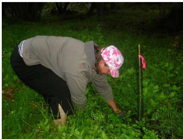
Figure 7. Water sample collection immediately downstream from bait. Bait was secured within a cylindrical wire mesh cage, and position marked with a bamboo pole and pink ribbon.
