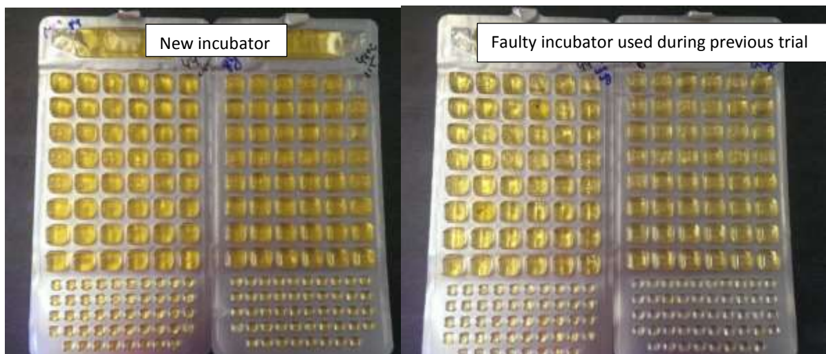
Figure D.25. Difference in the yellow colour generation (positive indication for total coliforms) for the same bacterial sample between two incubators used. The two quantitrays are for glycerol and previous trial E. coli stock.
