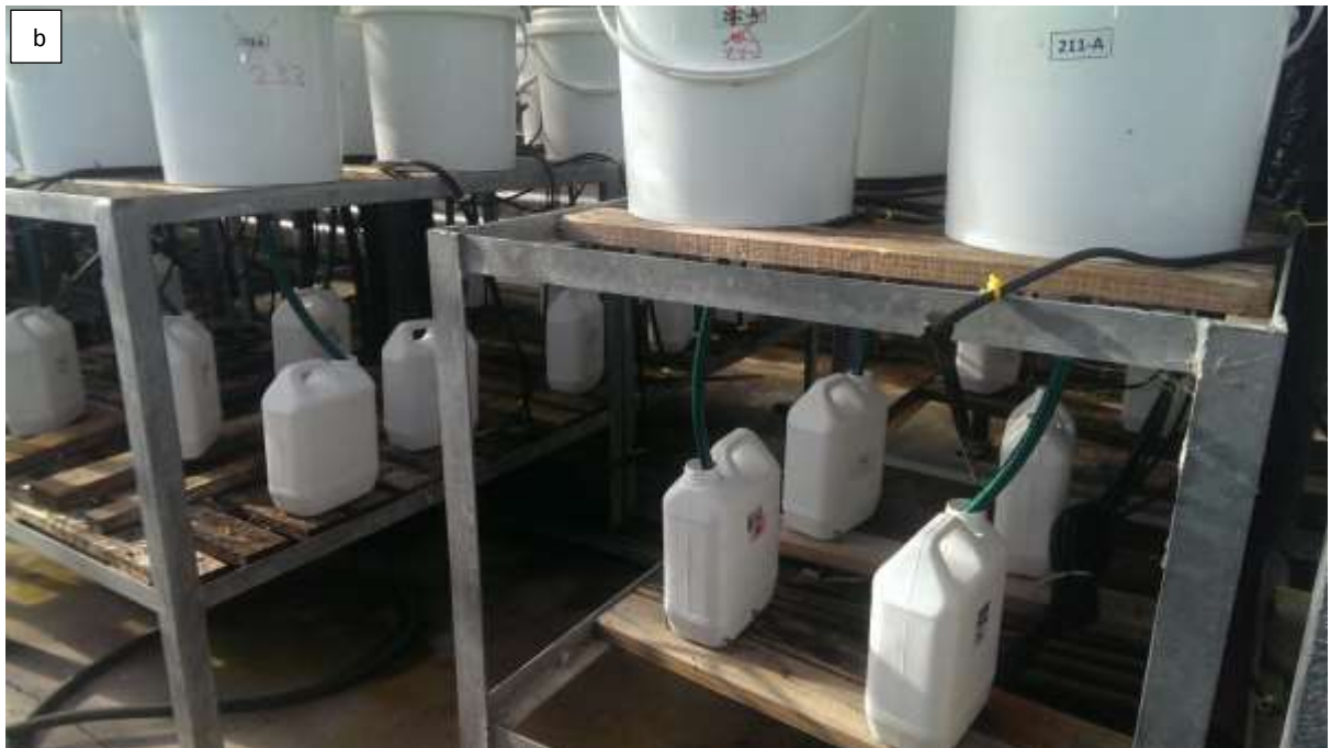
Figure 4-1 Shows a) experimental set up in the glasshouse and b) leachate collection.
