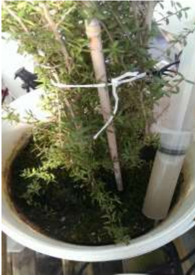
Figure D. 42. Petroleum jelly application on the sides of the lysimeters to seal the edges, avoiding preferential flow.
