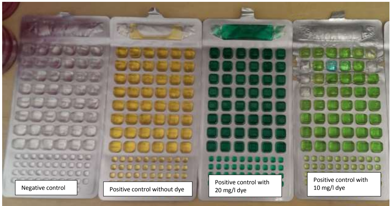
Figure D.39. Effect of Brilliant blue dye on the yellow colour production of Colilert at 36°C.
