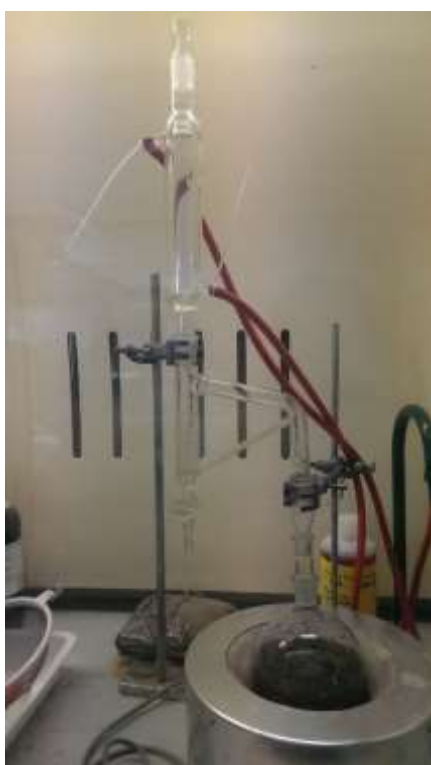
Figure D.17. The Clevenger set up for essential oil extraction.
