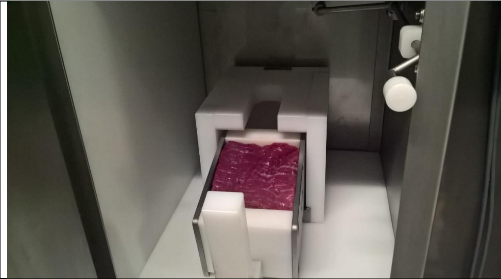
Figure 2.11 PEF treatment chamber in PEF machine
