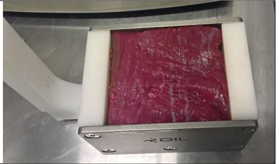
Figure 2.8 PEF treatment chamber with muscle block
