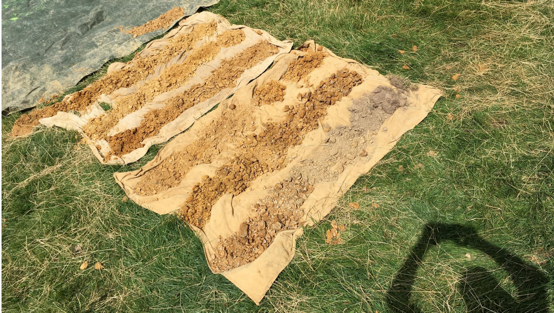
Figure A-1. Example of an auger boring (auger 2) between the topsoil (top of right-most column) and the gravels (bottom of left-most column), showing the change in colouring with depth.
