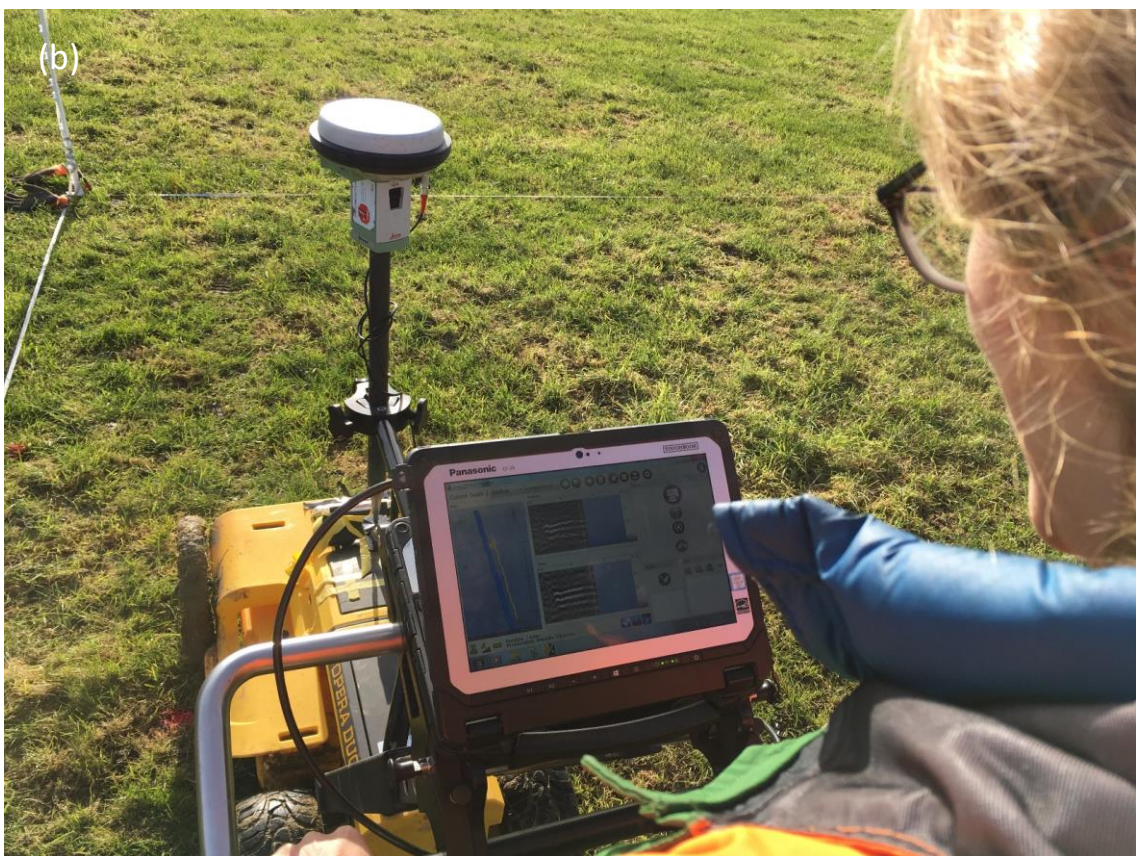
Plate 4-1. (a) Testing the ground-penetrating radar (GPR) device coupled with real-time kinematic (RTK)-GPS at the field site on a beautiful Southland evening. (b) GPR surveying of the mole channels in 10 x 10 m plots at high-resolution. The high-precision Leica Viva GS15 GNSS antenna is shown mounted directly over the radar. Real time reflections are shown on the screen and their locations recorded manually as a GPS coordinate at the apex of each reflector.
