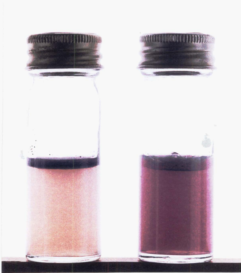
Figure 6.1: Degradation of cellulose by P. polymyxa 18:25 (right) but not by B. mycoides MW 27 (left).
