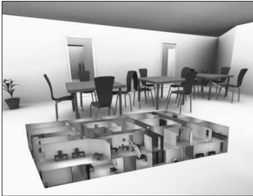
Figure 2-7 The The cut-away map according to the user's viewing direction in the VE (Andujar et al., 2010).
