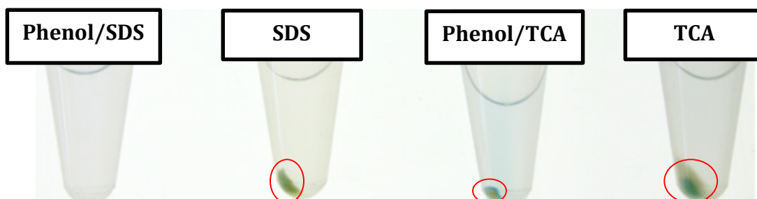
Figure 3.18. Protein pellet after precipitation with the precipitant and co-precipitants (2D Quant kit) were unable to be re-solubilised for protein content determination (indicated by red circles).
