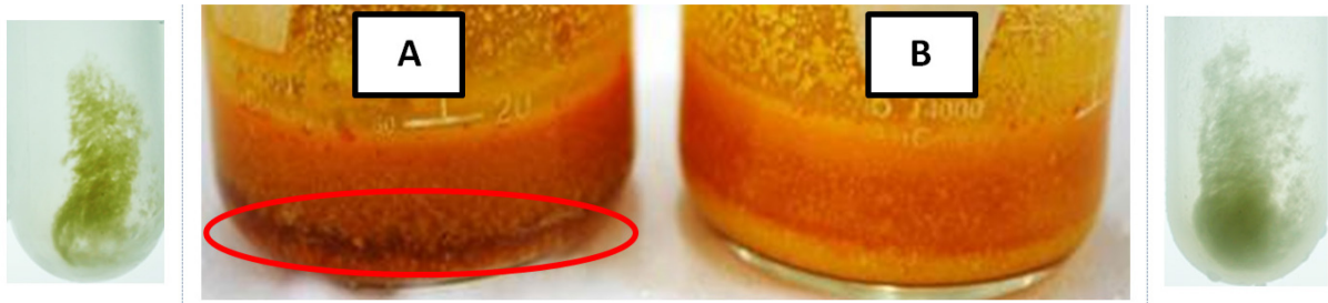
Figure 3.9. Re-suspension of mesocarps in buffered CDE after 6 hours incubation. A; without CDE, B; with CDE. A larger lipid layer is visible in A. Different sizes of chromoplast protein pellets are shown on the respective sides.
