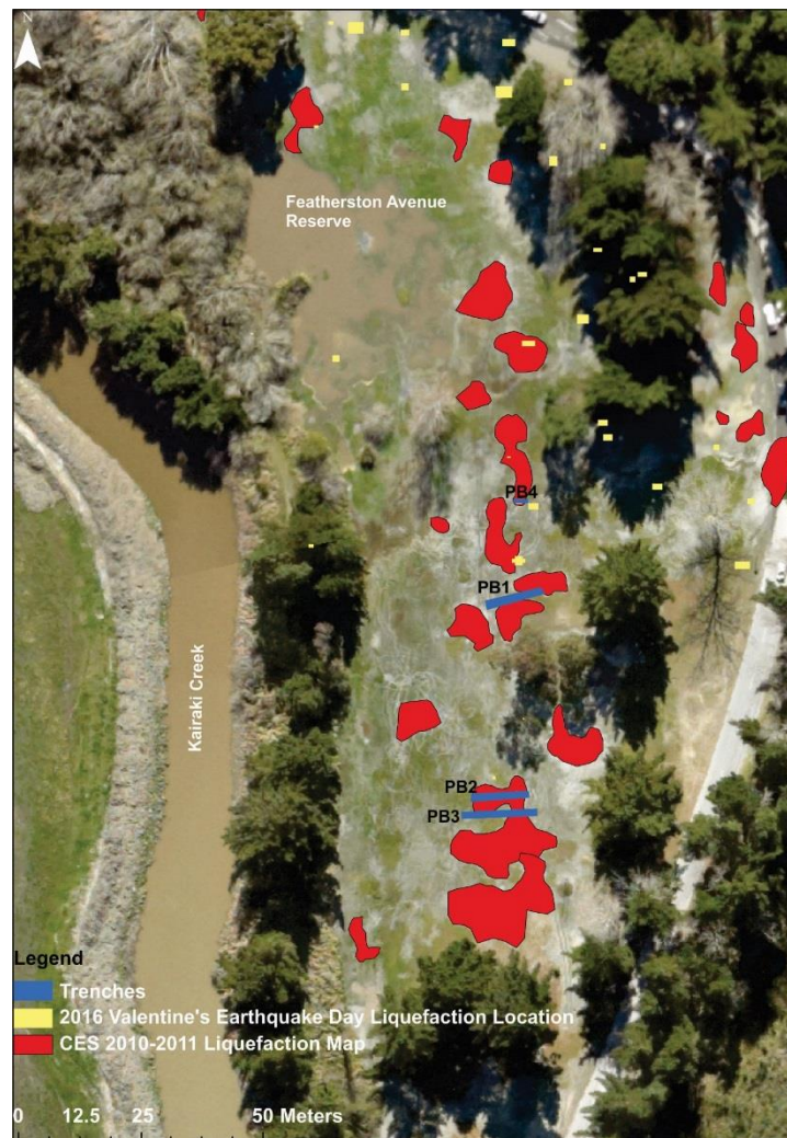
Figure 4. 3 Map of the liquefaction surface manifestation at Featherston Avenue Reserve caused by the 2010-2011 Earthquake sequence and by the 2016 February event. Location of paleoseismic trenches excavated before (PB1, PB2 and PB3 trenches) and after (PB4 trench) the Valentine's Day Earthquake.
