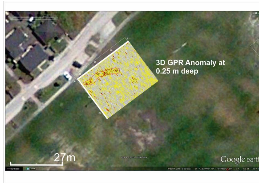
Figure 4. 7 3D GPR line at 0.25 m depth on Sand Blow1.
