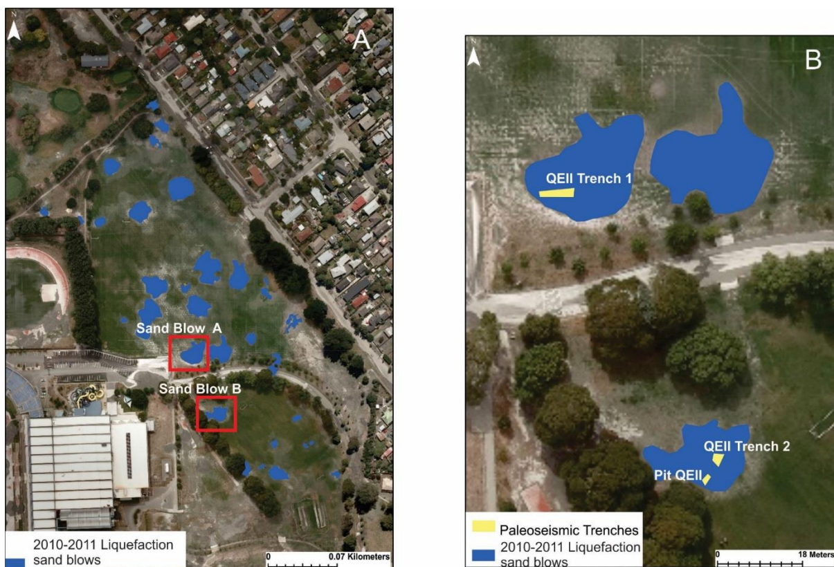
Figure 4. 4 QEII liquefaction mapping A) Sand blows targeted for the 3D GPR survey and trenching as a result of the 2D GPR survey; B) Trench locations on the targeted sand blow, QEII Trench 1 on sand blow A and QEII Trench 2 and Pit on Sand blow B. Please note the Pit QEII will be not described in this dissertation. Aerial photos from LINZ portal (LINZ, 2011).
