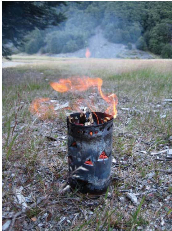
Figure 5.9e: Simple 'Twig Stove' made from a recycled tin can. Inside there is a raised plate so the base of the cooker does not overheat. 164
