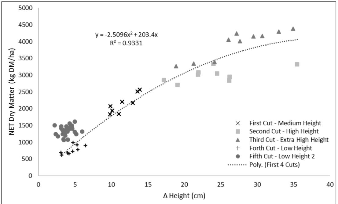
**Figure 4** Relationship between the device-measured change in height ( $\Delta$  Height) and net DM for Experiment 1.
