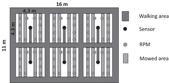
**Figure 1** Layout of Farmote device (sensor) testing stations and location of rising plate meter readings for preliminary investigations at the Lincoln University Research Dairy Farm.
