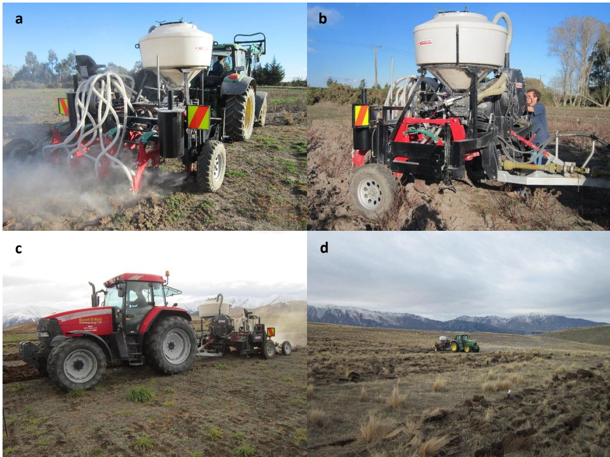
Plate 6.1 a. Rear view of the Flexiseeder lime ripper. b. Side view of the Flexiseeder lime ripper. c. Applying lime at the Omarama Station experimental site, 26 th May 2015. d. Applying lime at the Glenmore Station experimental site 25 th May 2015.
