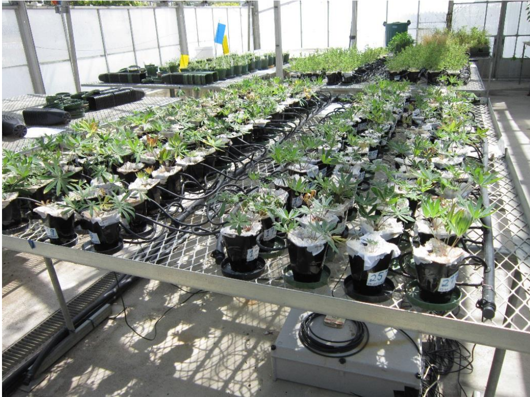
Plate 4.1 The automated irrigation system tubing in the Russell lupin pots. The data logger was stored in the grey box below the table.
