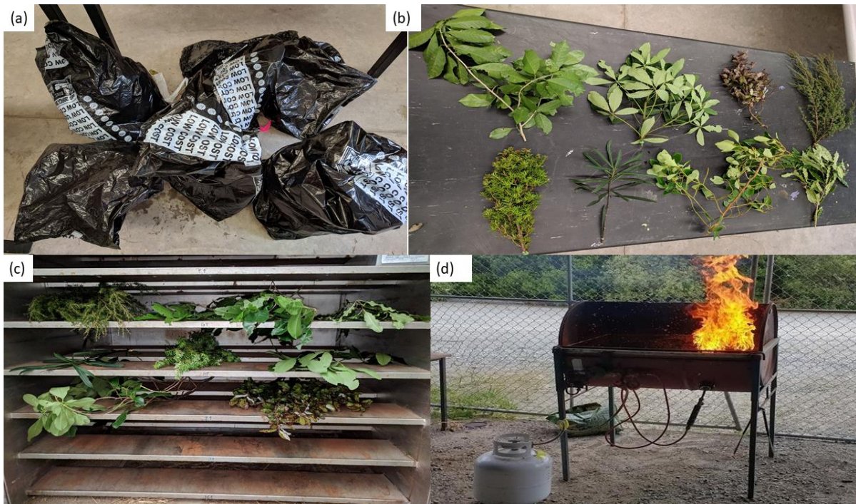
Figure 4.1. Wetting and drying treatments for samples and plant flammability device. (a) wet up treatments (plants with cut stems in water in darkness at room temperature), (b) air dry treatments, (c) oven dry treatment, and (d) apparatus for measuring shoot flammability.
