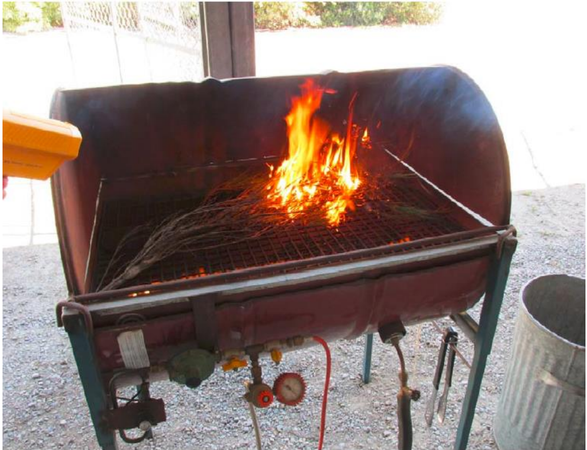
Figure 1.1 Device used to measure shoot flammability. A handheld infrared laser thermometer (left) is used to measure the flame temperature.
