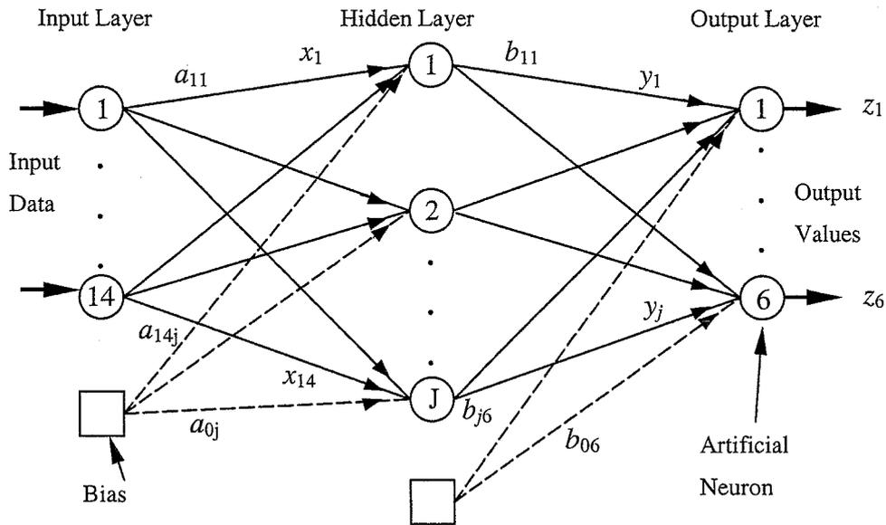
Figure 2. Three layer fully connected MLP network
