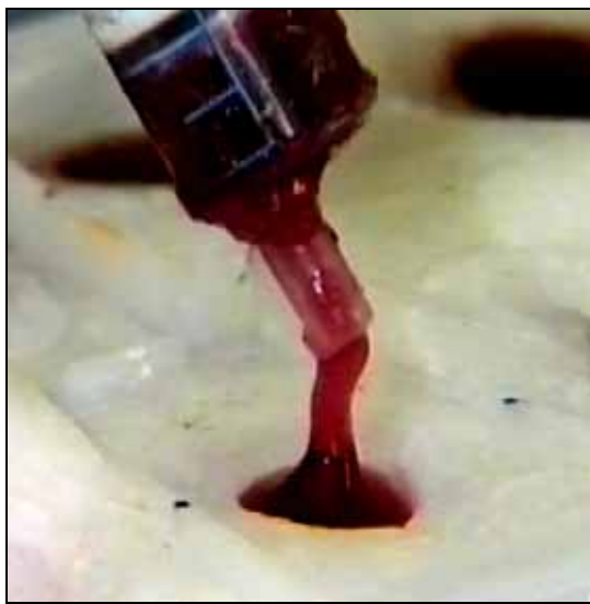
Figure 3.1 Piping the artificial grape mixture into a candlewax mould.
