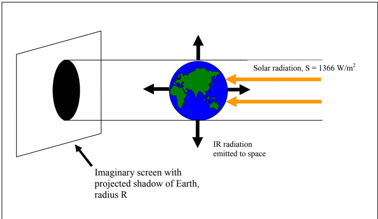
FIGURE 3. **Energy balance of Planet Earth.** Solar radiation ( $S = 1366 \text{ W m}^{-2}$ ), shown by incoming arrows, is intercepted over a circle (the ‘shadow’ area  $\pi R^2$  on the imaginary screen). Balancing this gain is a loss of infrared (IR) radiation (outgoing arrows), emitted from the *whole* surface of the sphere, area  $4 \pi R^2$ .
