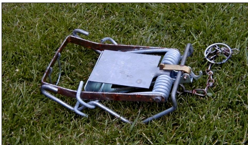
Figure 9. Fenn Mk 4 trap in set position (courtesy of Manaaki Whenua Landcare Research Ltd)
