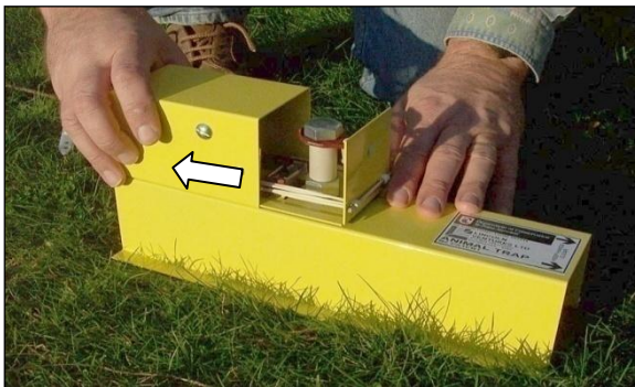
a) Here the cover has been slid back, thus loading the impact arm
