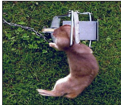
Figure 10. Fenn Mk 6 horizontal body strike on a stoat (courtesy of Manaaki Whenua Landcare Research Ltd)
