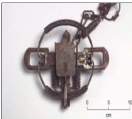
Figure 8. Victor No. 1 Soft Catch trap (courtesy of Manaaki Whenua Landcare Research Ltd)
