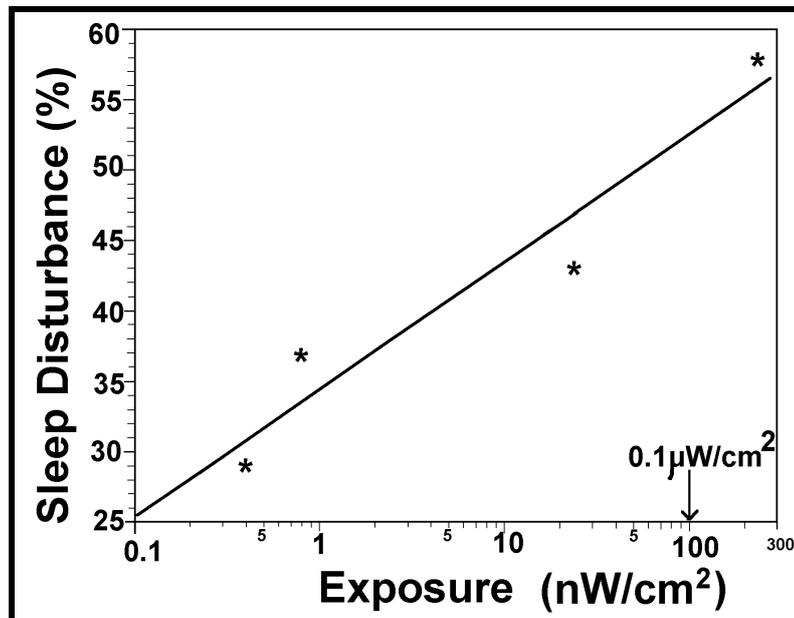
Figure 20: Dose-response relationship for Sleep Disturbance at Schwarzenburg with exposure in  $\text{nW/cm}^2$ . Note:  $1\text{nW/cm}^2 = 0.001\mu\text{W/cm}^2$
