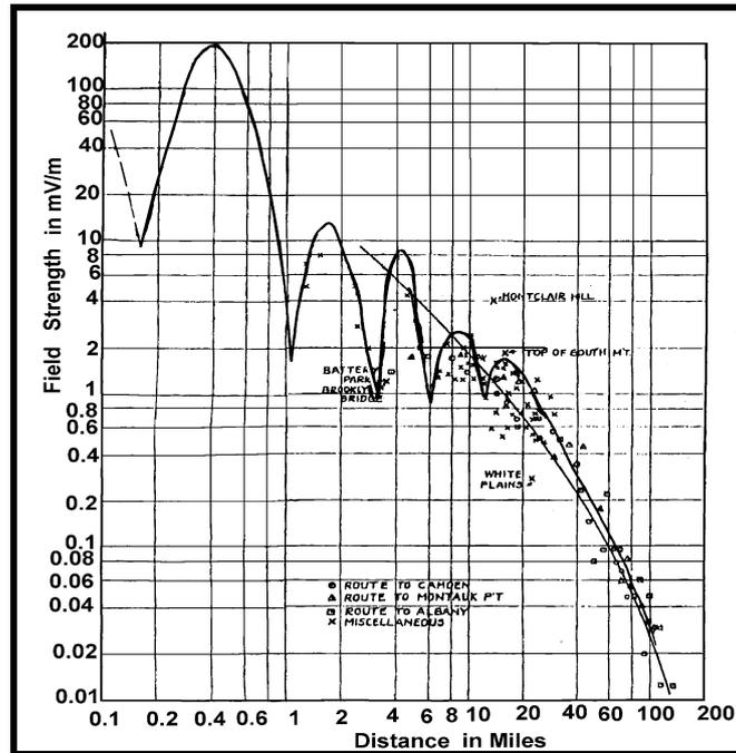
Figure 2: Ground level radiation pattern for (a) the 44 MHz (VHF) signal from the Empire State Building in New York City, from Jones (1933) by merging his figures 6 and 8,
