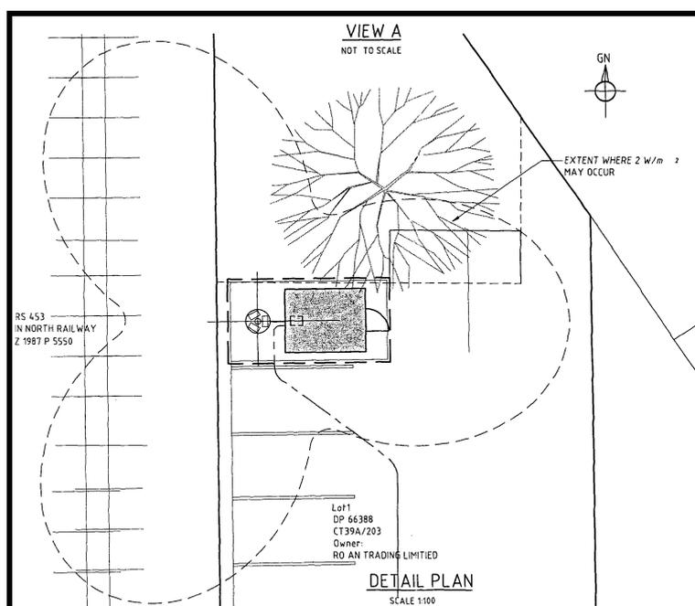
Figure 29: Three-panel horizontal radiation pattern, for a low powered site, as for the Elmwood Site.
