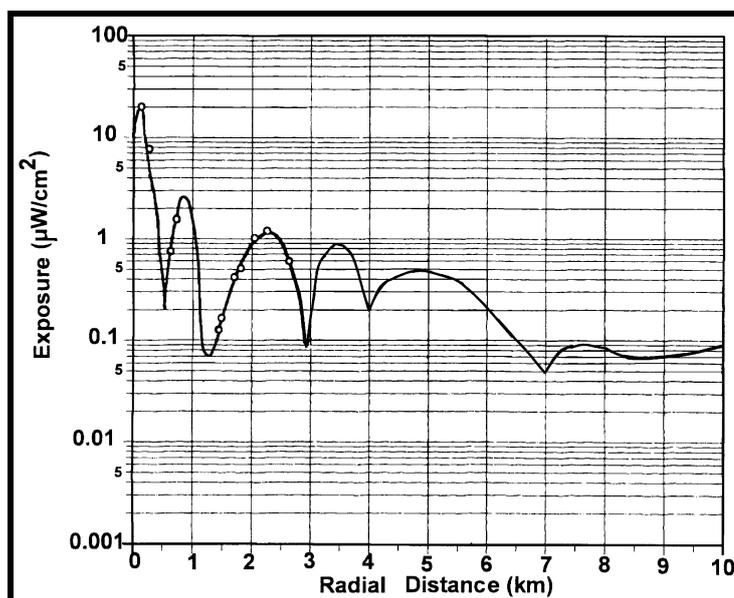
Figure 11: The measured and estimated power density (exposure in  $\mu\text{W}/\text{cm}^2$ ) with distance from the Sutra Tower. Circles show measurements. The line follows measurement points and the radial pattern of Figure 6 beyond 3 km. From Hammett and Edison (1997) and readings taken by the author in 1999.
