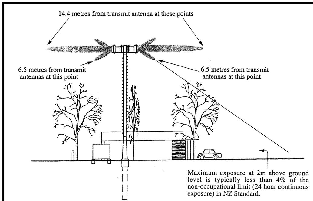
Figure 26: Cell site profile showing the extent of the main beams and side lobes in which the  $200 \mu\text{W}/\text{cm}^2$  standard is exceeded. This illustrates the directions of the beams and side lobes.
