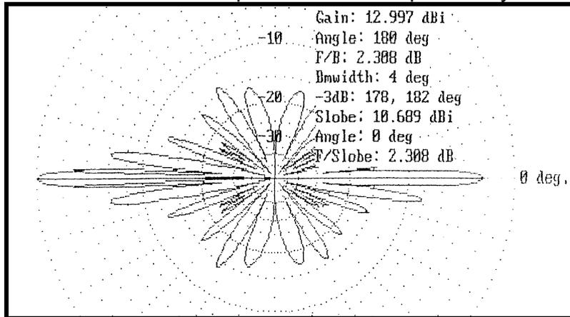
Figure 4: A typical vertical antenna pattern for a 4-element dipole array at about 98 MHz.(VHF), Units in dB.
