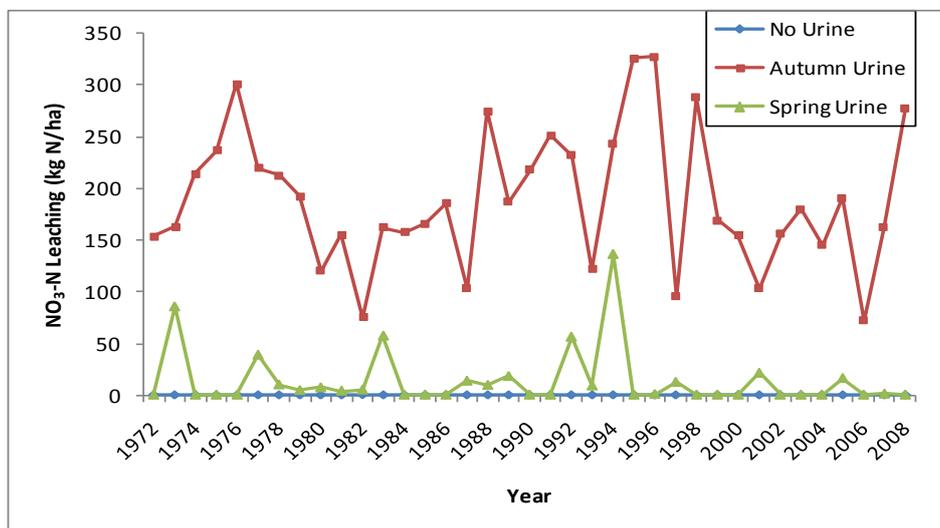
Figure 4: Average  $\text{NO}_3\text{-N}$  leaching under autumn-applied, spring-applied, and nil urine for each year from 1972 to 2009.
