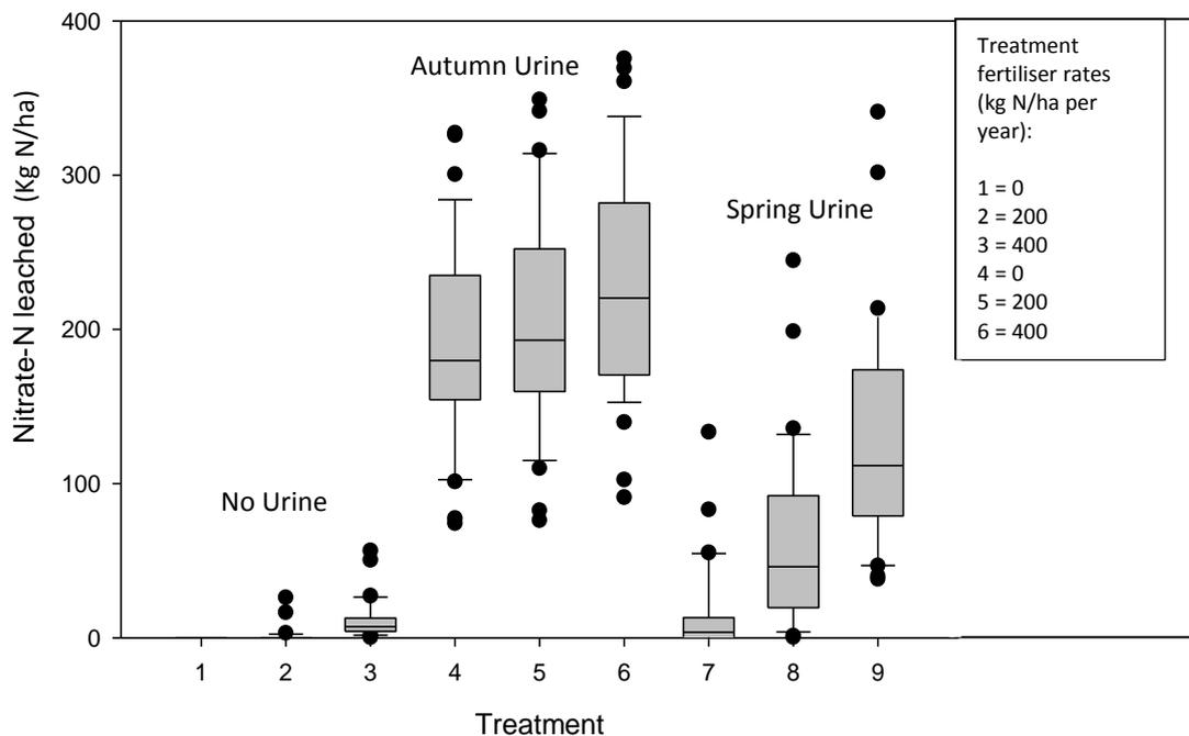
Figure 2: Box plot showing average NO<sub>3</sub>-N leaching over 37 years (1972-2009) for three different fertiliser rates applied with three different urine applications (nine treatments in total).
