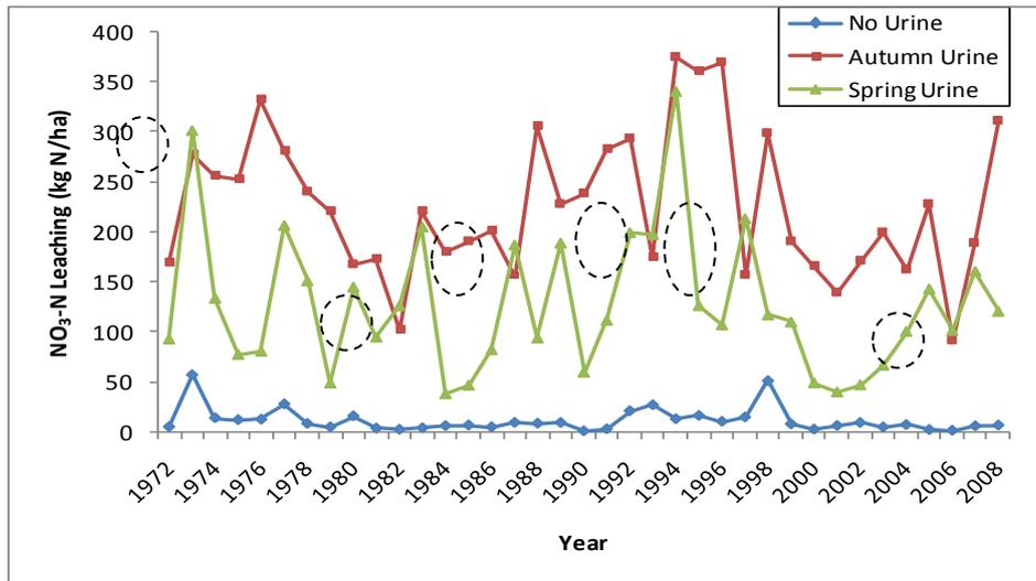
**Figure 5: NO<sub>3</sub>-N leaching under fertiliser rate of 400 kg N/ha plus autumn-applied, spring-applied or nil urine. The circled points denote the years where modelled leaching under spring-applied urine was greater than under autumn-applied urine.**
