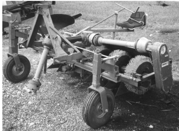
Figure 5. Horizontal axis brush hoe
