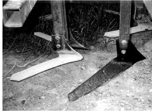
Figure 4. Poorly designed hoe blades
