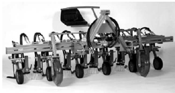
Figure 7. Vertical axis brush hoe
