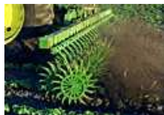
Figure 2. Spoon weeder / rotary hoe
