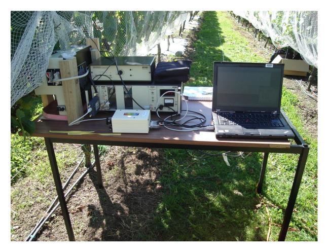
Figure 3. 3 – Bentham spectroradiometer reading reflection data
