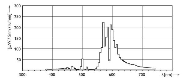
Figure 3. 5 – Photometric data of the bulb used in the trial (MASTER SON-T PIA Plus 600W/220 E40 1SL)
