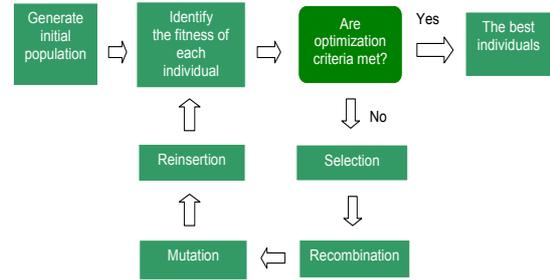
**Figure 1:** Structure of a single population Genetic Algorithm
