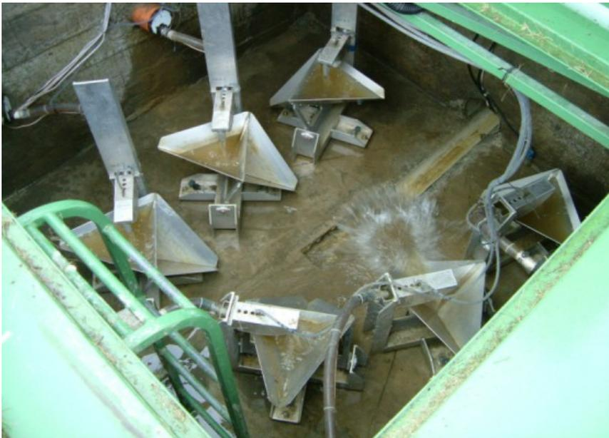
**Plate 3.** Simultaneous measurement of the drainage rate from six plots by the tipping bucket method
