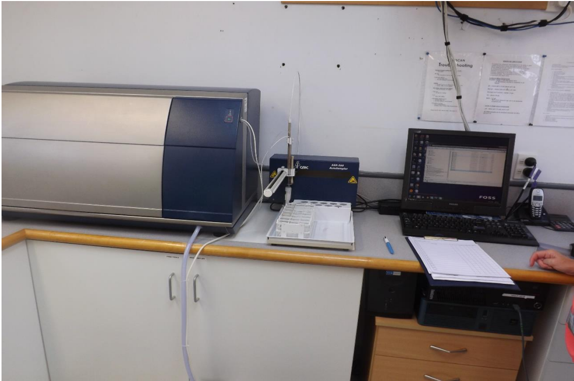
Figure 4.3. Measurement of maturity indices. A. Grape berries sampled into a zipped plastic bag; B. Juice from crushed berries; C. WineScan WineScan™ FT 120.
