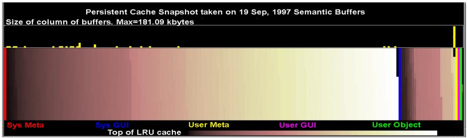
Figure 1 b. Display of the persistent cache from the test snapshot with buffers grouped according to their semantic type (system meta object, system GUI object, user meta object, user GUI object, user object, user object).
