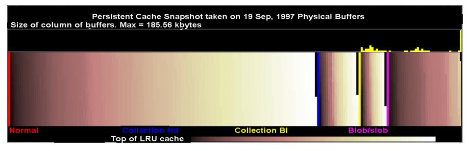
Figure 1 a. Display of the persistent cache from the test snapshot with buffers grouped by their physical type (normal, collection header, collection block, blob/slob).
