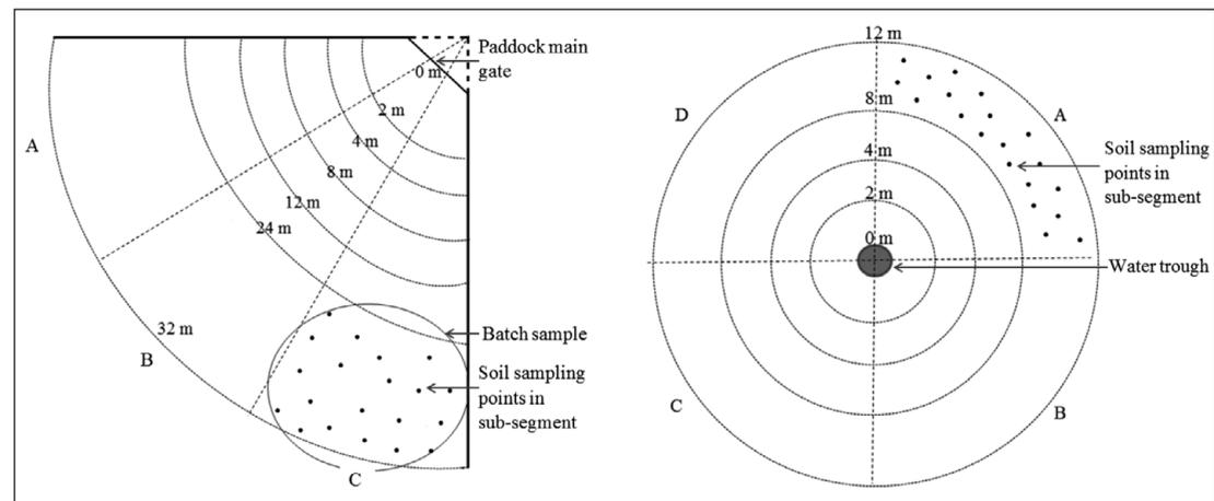
Figure 1 Illustration of sampling procedure at paddock main gate (left) and around water trough (right).
