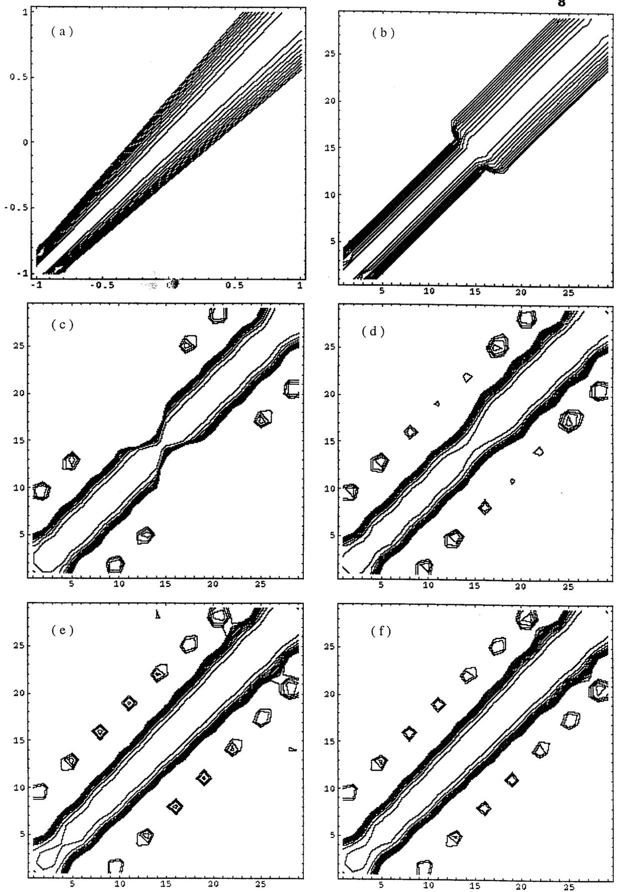
Figure 4: Contour plots of various representations of the exponential covariance function. a) Exact kernel b) stepwise kernel c) 9-term PE expansion d) 9-term PKM expansion e) 9-term DCLM expansion f) 9-term exact eigenfunction expansion
