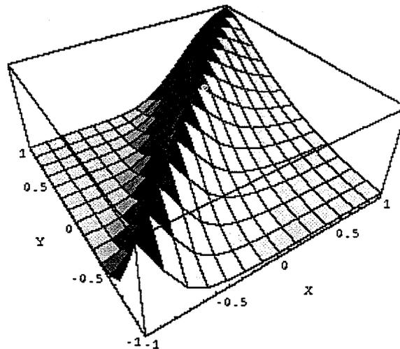
**Figure 1:** Schematic view of a variable correlation length covariance function;  $\lambda$  increases in the direction away from the viewer.
