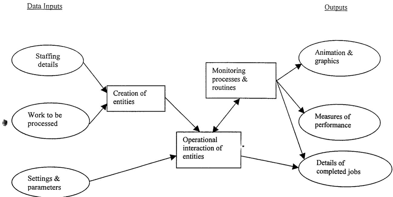
Figure 1: Schematic diagram of conceptual model. Throughout execution the model's state records to file. Inputs and settings are supplied from computer files, while measures of delay and performance are both recorded to file and displayed using animated graphics.
