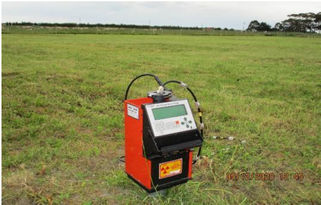
Plate 3.4 Soil profile moisture measurement (2.2 m) by Neutron probe (CPN 580) in Iversen 8 experimental site at Lincoln University, Canterbury, New Zealand.
