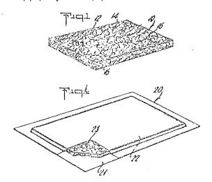
(57) The product 10 comprises bleached peat moss 12 and finely divided mechanical wood pulp 14 having a Canadian Stronbard Freeness Value of from 30 to 600 and present in a ratio, by weight of the wood pulp to the peat moss, of more than 0.35. The product may include long-fibered absorbent material 16 such 4s rayon fibres. The product may be used as an absorbent core 23 disposed between a fluid impervious backing sheet 21 and a fluid pervious facing sheet 22 of a disposable diaper 20.
