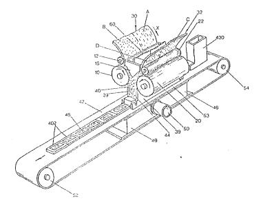
(57) An air laid fibrous product 45 is made by fiberising two fibrous materials 30,32 in lickerins 10,20. The resulting loose fibres are drawn by an air current 44 into molds 402 carried on conveyor 42. The molds have their bottom part formed as a screen, while the conveyor is also formed from screen material, so that air may be drawn through the mold and conveyer. By moving a separator into mixing duct 40 the relative distributions of the two types of fibres in the mold may be varied.
