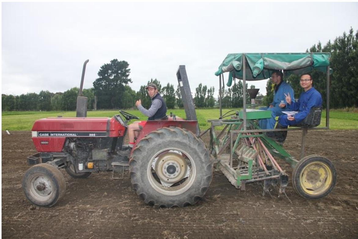
Plate 4.2 Sowing the lucerne seed in the field with cone seeder
