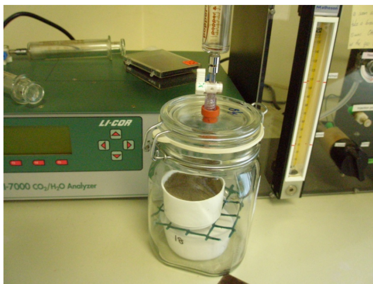
Figure 4. Collection of gas samples (infrared gas analyser in the background).
