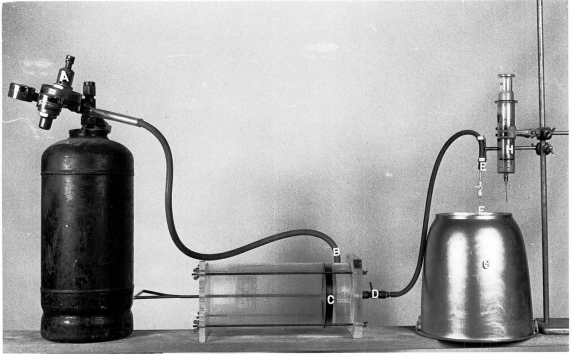
Plate 3.1: Acetylene reduction apparatus for *in situ* measurement of nitrogen-fixing activity.
