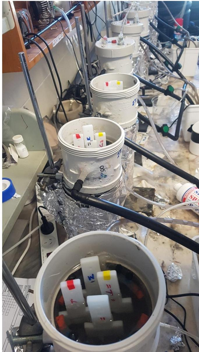
Figure 3-4 The arrangement of DGT and DET probes during deployment in mesocosm.
