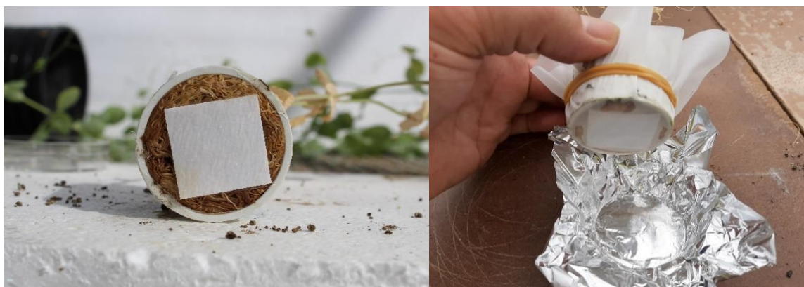
Figure 2.2 The method of rhizoplane organic anion collection by anion exchange membrane.
