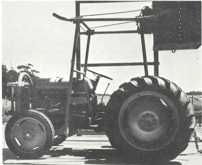
Fergrac safety frame after impact from rear.
