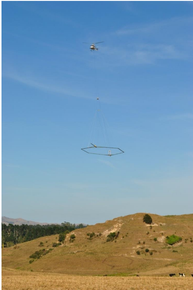
Fig. 4: The SkyTEM system carrying out the helicopter-borne electromagnetic survey of the Piako River headwater catchment, February 2019.
