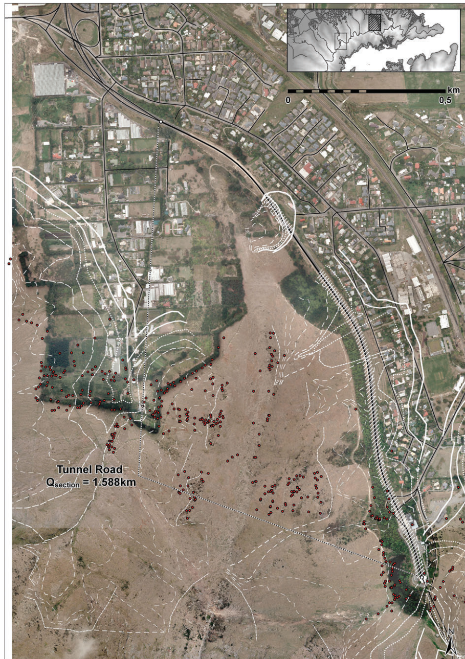
Figure 4 Shadow angle lines (in white) depicting maximum rockfall runout on Tunnel Road (black dots: mapped boulders of the 2010/2011 earthquake sequence). Sources: Land Information New Zealand 2015, CCC n.d.
