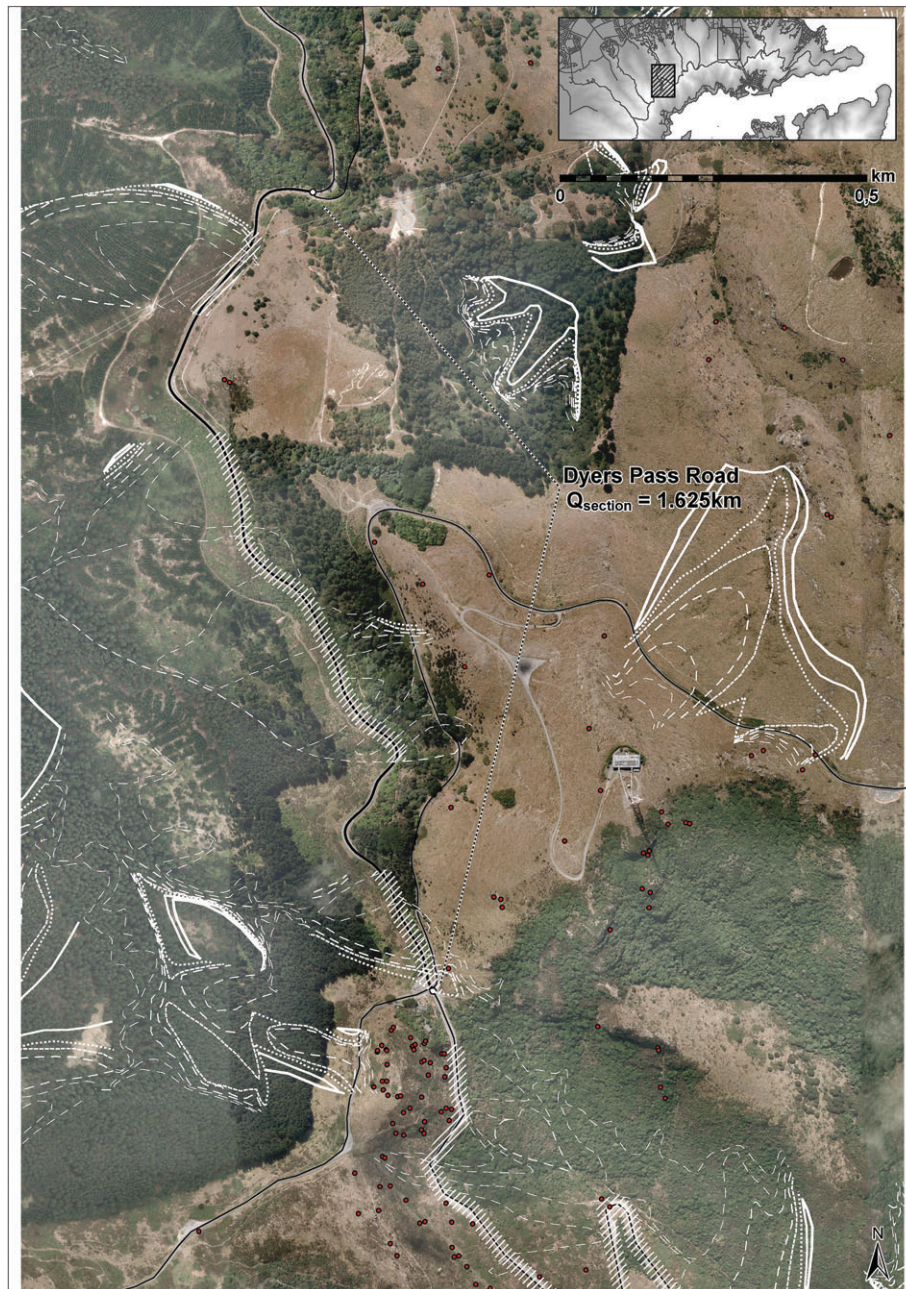
Figure 5 Shadow angle lines (in white) depicting maximum rockfall runout on the studied section of Dyers Pass Road (black dots: mapped boulders of the 2010/2011 earthquake sequence). Sources: Land Information New Zealand 2015, CCC n.d.
