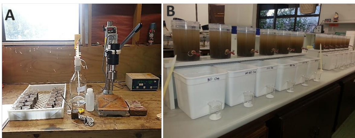
Figure 3.5. A) Ultrasonic probe for soil dispersion before the particle size fractionation, B) Soil size particle fractionation by gravimetric method using calcium chloride dehydrate as a flocculent to promote settling of clay soil particles (< 5 \mu\text{m} ).
