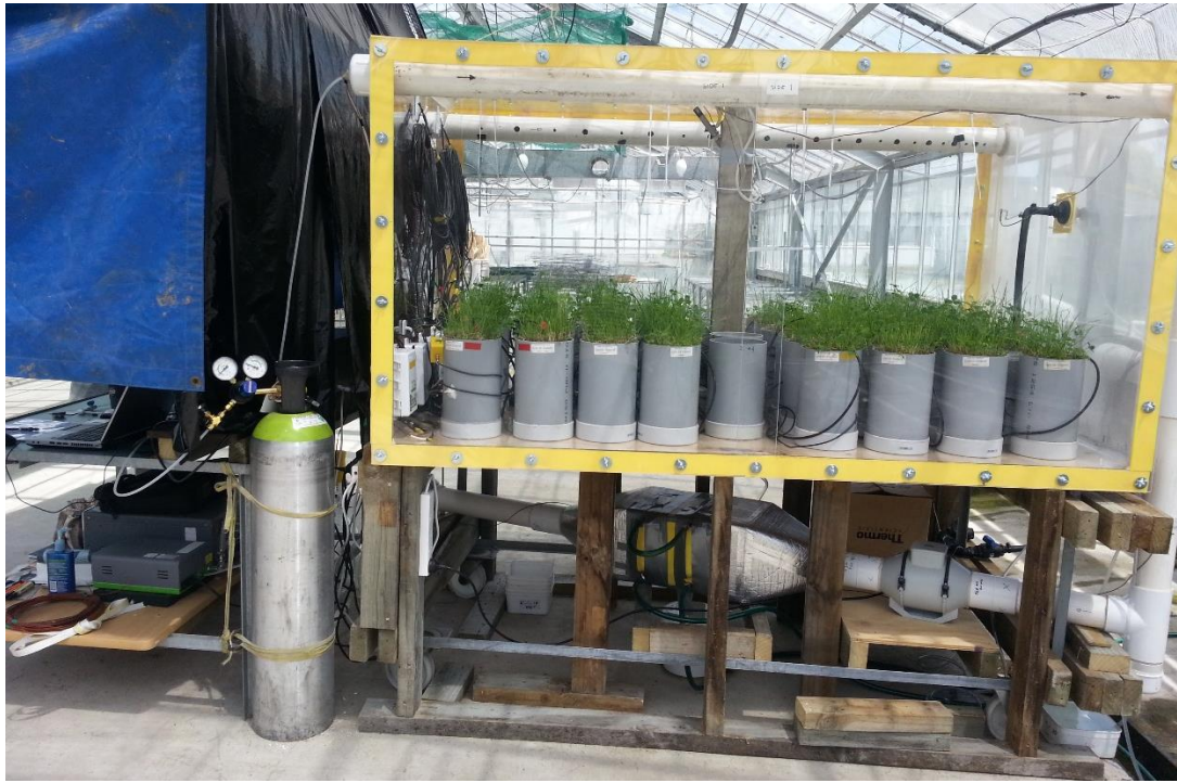
Figure 3.3. Plant growth chamber for ^{13}\text{CO}_2 labelling. The heat exchange unit can be seen under the chamber. The side wall panels are removable for easy access to the mesocosms. The addition of ^{13}\text{CO}_2 and ^{12}\text{CO}_2 into the chamber was controlled by a gas isotope analyser (Picarro).
