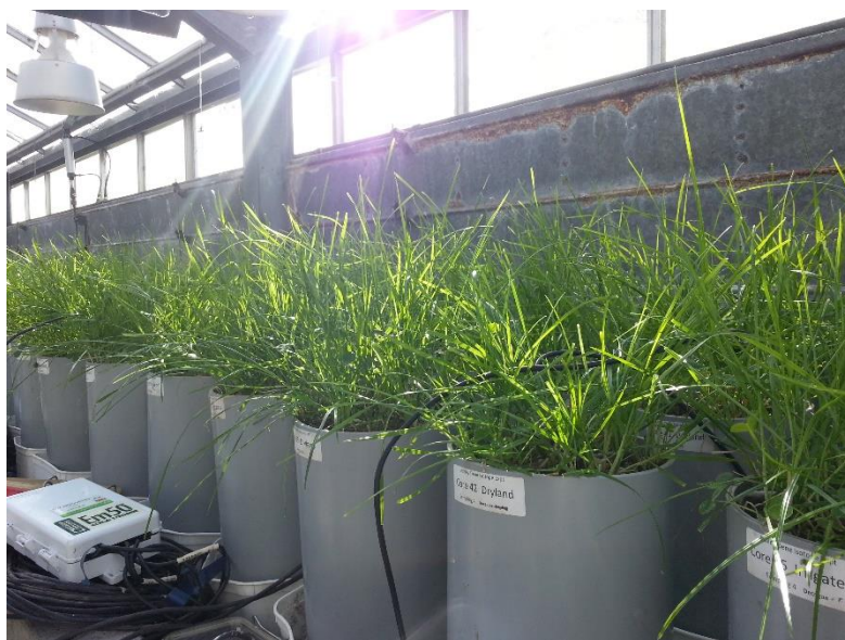
Figure 3.2. Ryegrass-white clover established mesocosms with connected Decagon soil moisture sensors.
