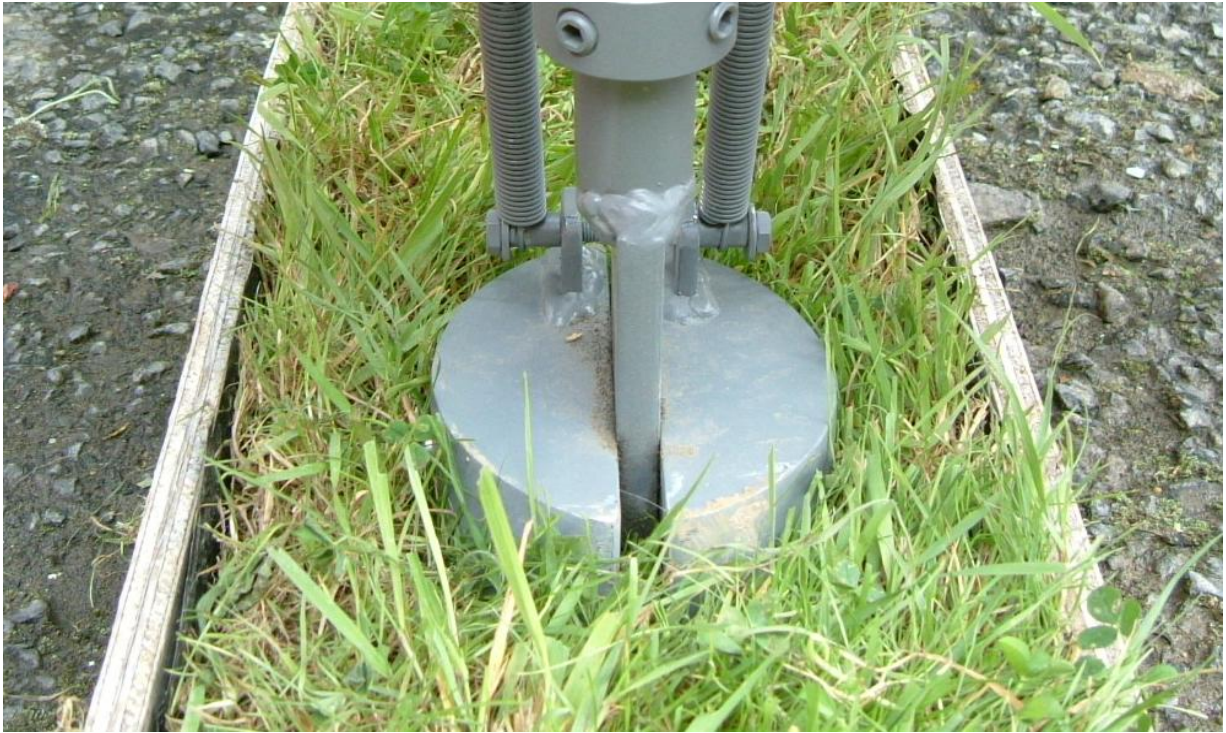
Figure 3.1. The mechanical cow hoof simulating treading on an excavated block of soil.
