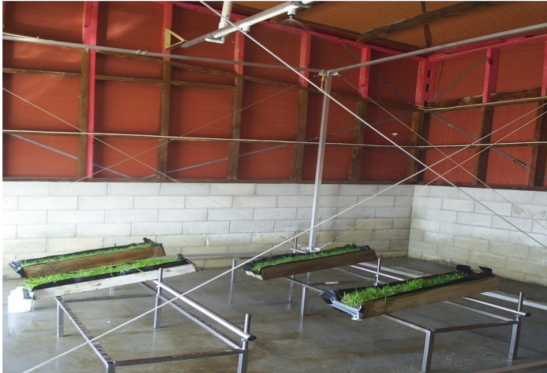
Figure 3.2. Rainfall simulator set up to create surface runoff from treaded upon soil blocks.
