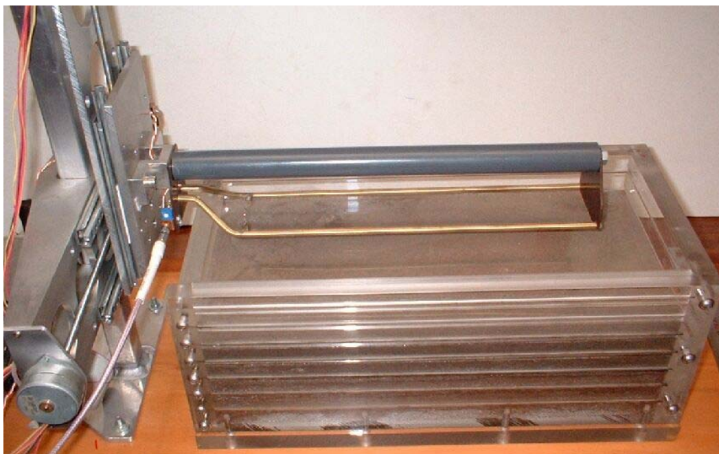
Fig. 2. Arrangement of the waveguide and the physical model of a layered soil profile. The apparatus at the left enables adjustment of the y -axis (vertical position) of the waveguide.
