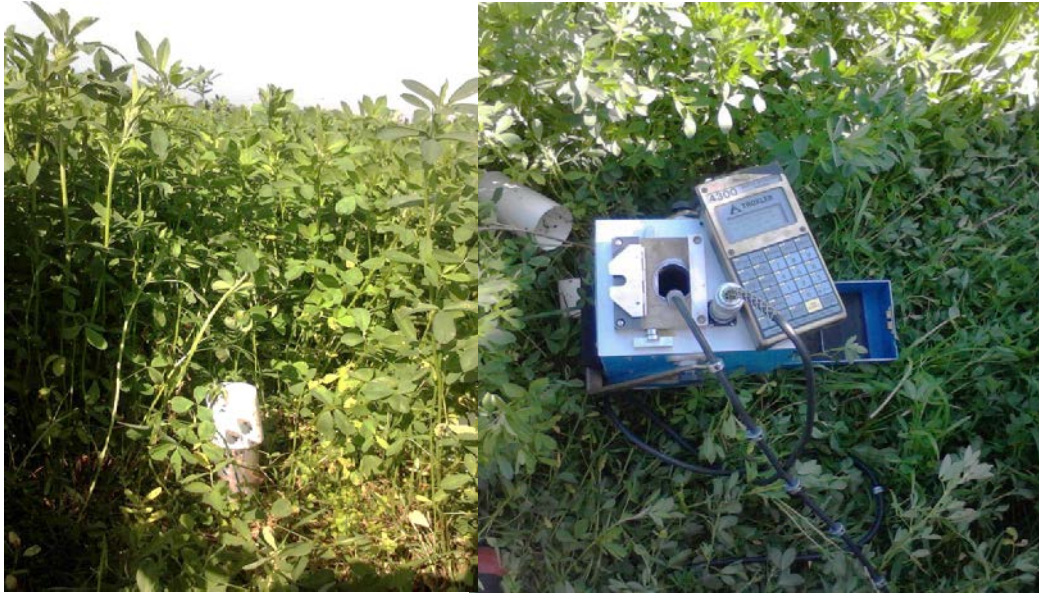
Plate 3.2: Measurement of soil water content with a neutron probe (Troloxler) in Plot 1 at Ashely Dene, Canterbury on 27/03/2014.
