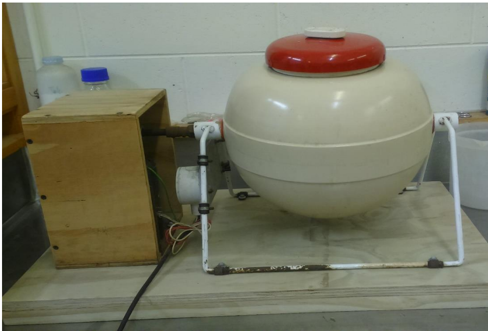
Plate 3.2 Modified hand operated washing machine (Banmix Food Machine Ltd., Auckland, New Zealand) used for washing larvae from the grass samples.
