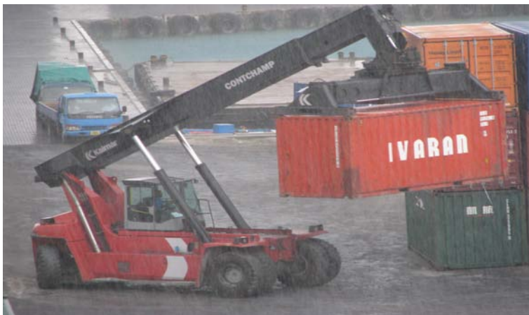
Figure 2.6: Reach-stacker at Male' Port, Maldives
