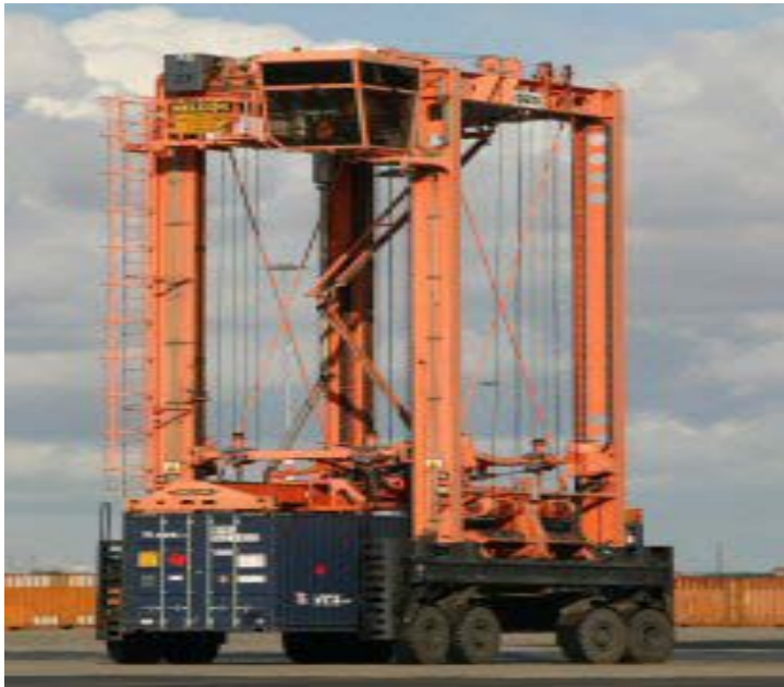
Figure 2.5: Straddle Carrier at Amsterdam Container Terminals, the Netherlands
