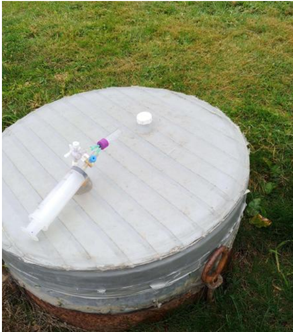
Figure 3-10. Gas chamber atop drainage model unit with syringe and 5 mL vial.
