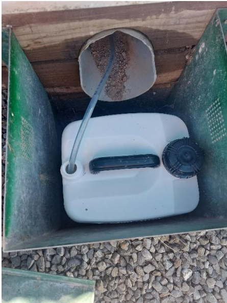
Figure 3-5. Clean plastic tube and container attached to the drainage nipple at the base of each drainage unit and used to collect the drainage water samples.
