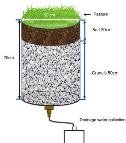
Figure 4-1. Design of cylindrical drainage model used in study (Che et al., 2022).
