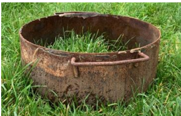
Figure 3-2. Metal cylinder used to obtain topsoil layer.
