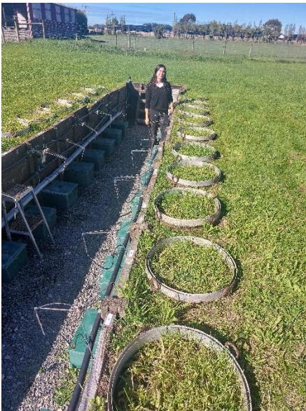
Figure 3-4. Trench with the drainage model units installed.
