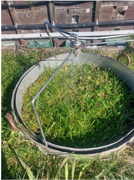
Figure 3-6. Rain/irrigation simulation system placed on top of lysimeters.
