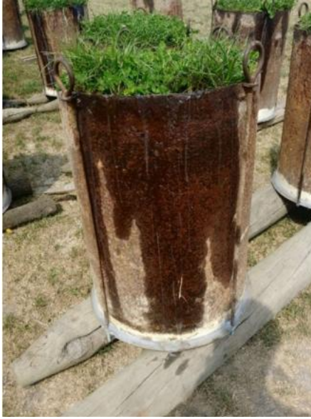
Figure 3-3. Final drainage model unit with gravel and topsoil layers before installing into the trench facility.
