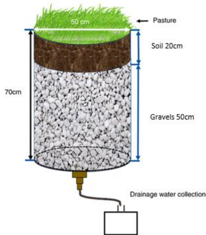
Figure 3-1. Design of cylindrical drainage model used in study (Che et al., 2022).
