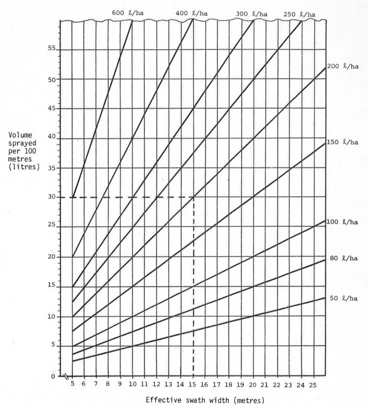
Example (see dotted line):- A sprayer with a swath width of 15m at 200  $\mbox{\&/ha}$  should deliver 30 litres in a 100m run.
