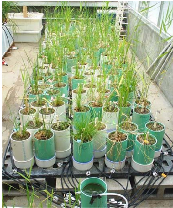
Figure 2: The columns and water replenishment system at MSU (Stein, 2012).
